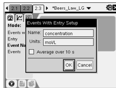
12. When the value displayed on the screen has stabilized, click the **Keep**
