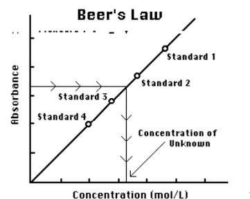
The concentration of an unknown  $\text{NiSO}_4$  solution is then determined by measuring its absorbance with the Colorimeter. By locating the absorbance of the unknown on the vertical axis of the graph, the corresponding concentration can be found on the horizontal axis (follow the arrows in the figure to the right). The concentration of the unknown can also be found using the slope of the Beer's Law curve.
